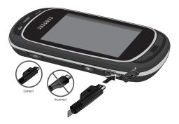
Note: The previous illustration displays the incorrect method for connecting the charger. If attempted, damage to the accessory port will occur therefore voiding the phone's warranty.
